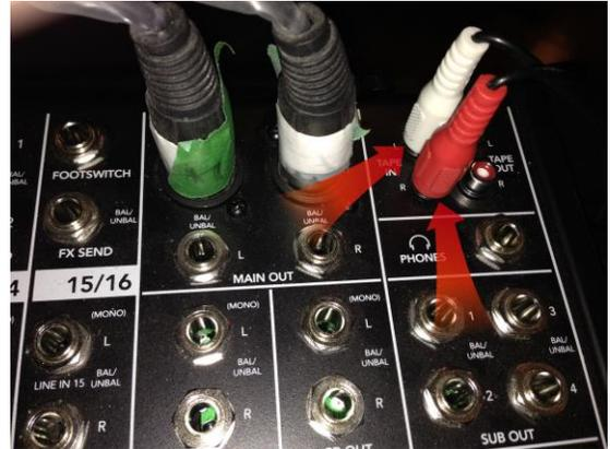
Using a 3.5 mm Audio to RCA Audio Cable, attach one end to the positions on the Mackie Mixer (red on red and white on white) and attach the opposite end to the source device. The volume control for these inputs is located on the Mackie Mixer as shown below.
